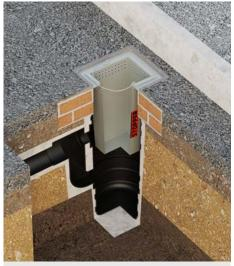
Place more mortar above the MuckStopper frame and complete the installation of the gully grating and frame per the manufacturer's guidelines above the MuckStopper. During installation of the gully grate, ensure the bucket is positioned correctly for removal.
