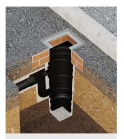
Before installing the gully grating & frame, install the MuckStopper above the brickwork. Bed the MuckStopper frame in place with mortar and ensure it is level. Ensure the narrow side of the frame is against the kerb.
