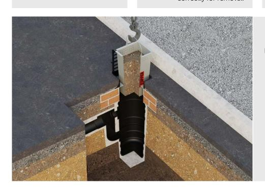
The MuckStopper should be extracted using machine lift. At the end of the project, the MuckStopper should be removed. The grating and frame can then be reinstalled when setting final levels before surfacing as usual.
